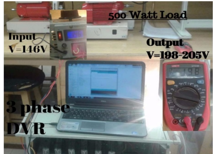
Figure 19: Testing of three phase DVR in the laboratory with a single phase load
